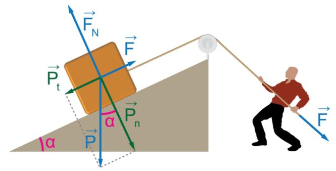
And this would be a still more generic case in which an inclined plane, a string and pulley is used.
